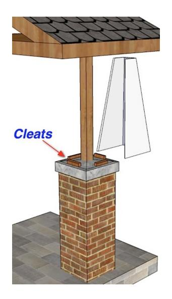
7. Install pin or screw this U section to the cleats. Others suggested that two "L" shaped pieces should be assembled but we find using the U method easier as trees or shrubs are less likely to get in the way.
