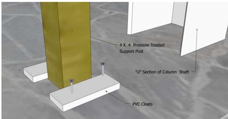
4. Fasten using Tapcon Screws, staples, pins, and/or adhesive the enclosed PVC cleats to the bottom of the shaft, direct contact with concrete is acceptable. For the top, use Pressure Treated Lumber cleats(not included).
