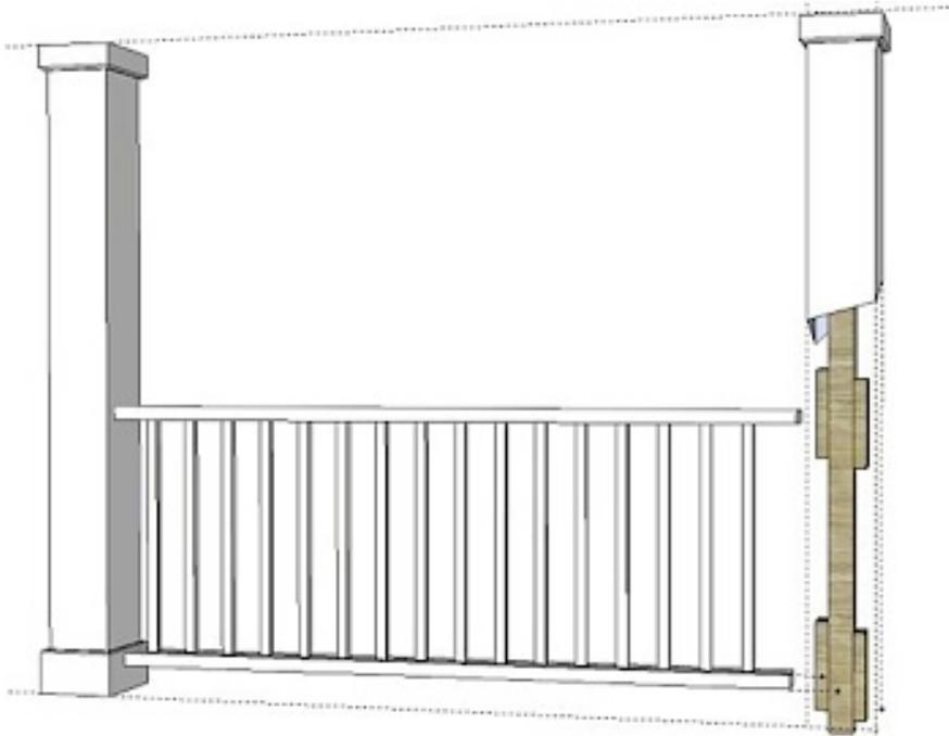
**Railings:** If there are railings to be installed, insure the rails are secured to the structural support. Use only code approved methods for installation. Use a metal bracket or pressure treated lumber the thickness of the space between the support post and the inside of the PVC wrap. Do not use un-treated lumber for structural or railing support.
