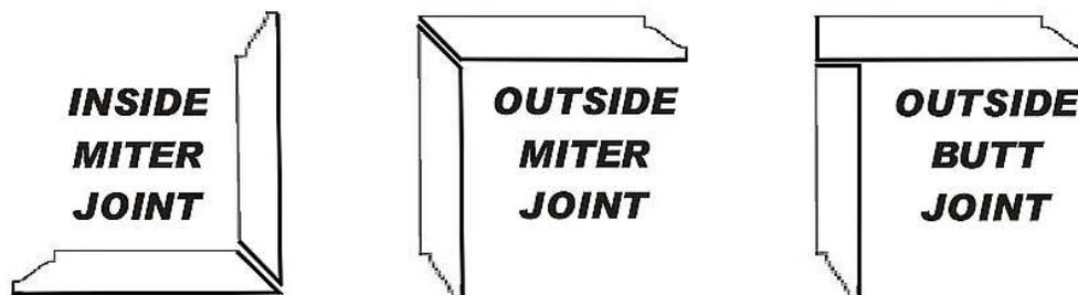
The butt joint method will work just as well, but allow a little more time to sand down the seam. If you still see a slight seam, don't feel bad, walls are rarely square. A little spackling or caulking is all it takes to fill these slightly larger seams.
