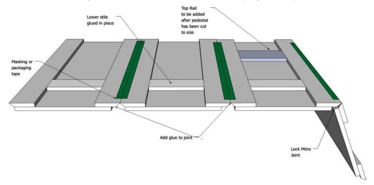
\*The process of taping together column panels, applying adhesive to 90 degree or lock mitre joints, then rolling and folding them into shape is called the book tape method. This method makes a very tight seal, which results in a strong bond. Test to make sure that the panels are square then fasten with an air stapler or brad nailer.
