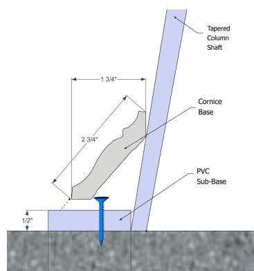
Tapered columns, less than 6ft, are often installed on pedestals. However, taller columns (over 6ft) are often mounted directly on the concrete floor. When installing the wrap on the concrete floor, we provide an additional PVC Sub-Base. This additional support helps to withstand impacts such as snow shovels and foot traffic.
